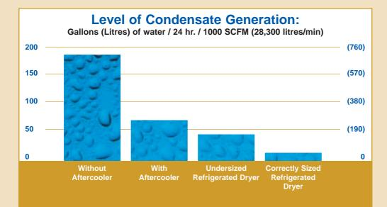
A 100 HP (75 kW) compressor operating with an aftercooler for 8,000 hours a year will produce over 10,000 gallons (38,000 litres) of condensate, enough to fill a swimming pool. The good news is most waste water regulators accept direct discharge of condensate from compressors running with Ultra Coolant.
